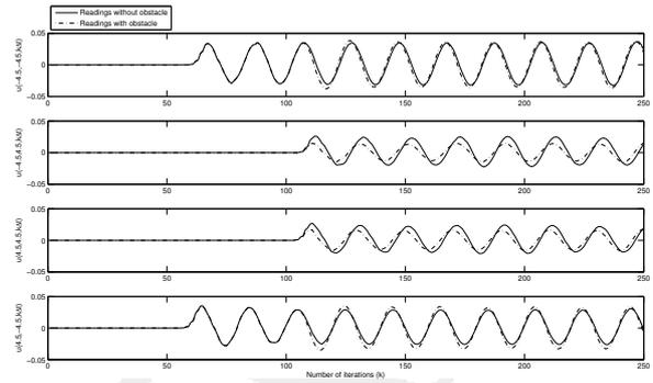
Fig. 3. Sensor readings - nominal readings without object in sound field (solid line), or with object in sound field (dashed line) .
