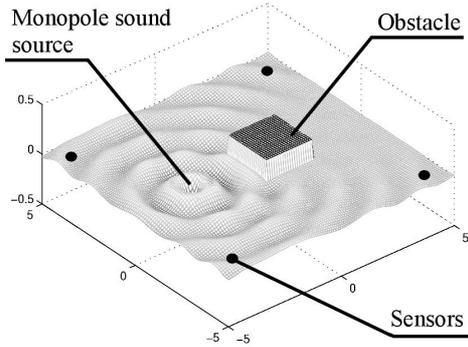
Fig. 2. Sound source and obstacle
