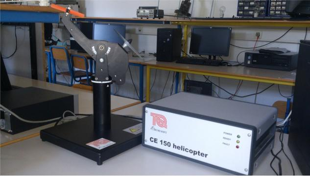
Fig. 4. Laboratory helicopter system Humosoft CE 150
