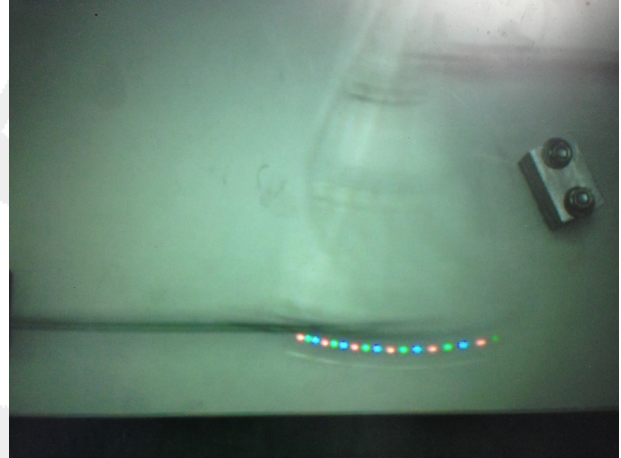
Fig. 1. Frame taken while moving the proposed modulated active marker - 2FPS, 500ms exposure time
